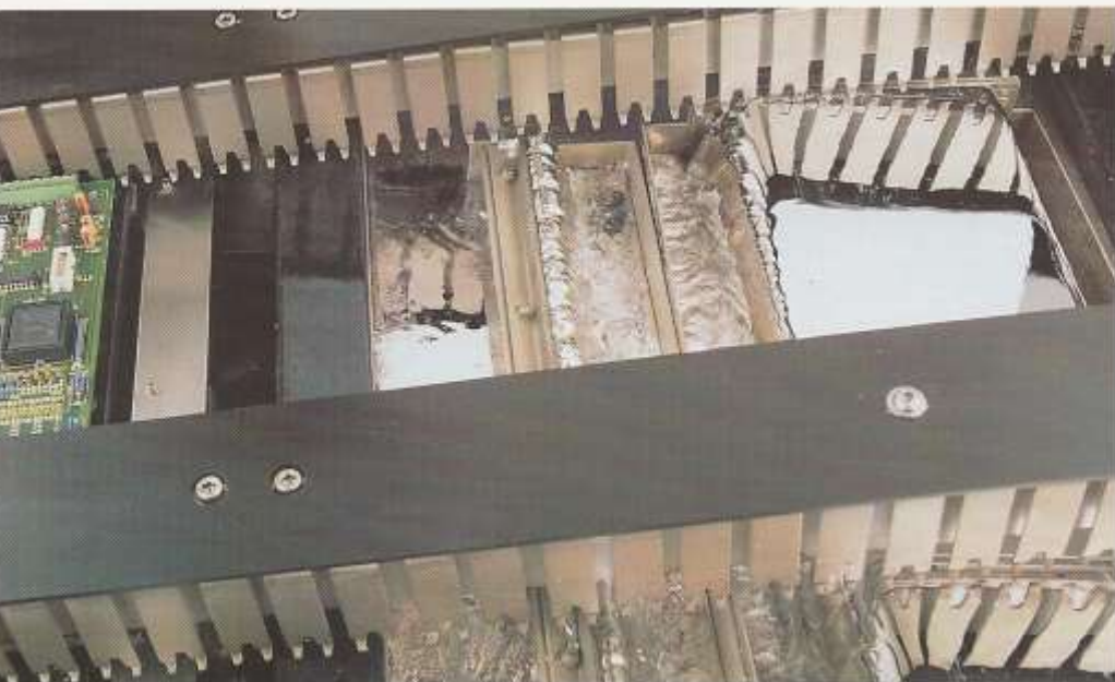
▼ Jet wave and laminar wave dual solder bath The roll-out pot makes servicing much easier ▼
